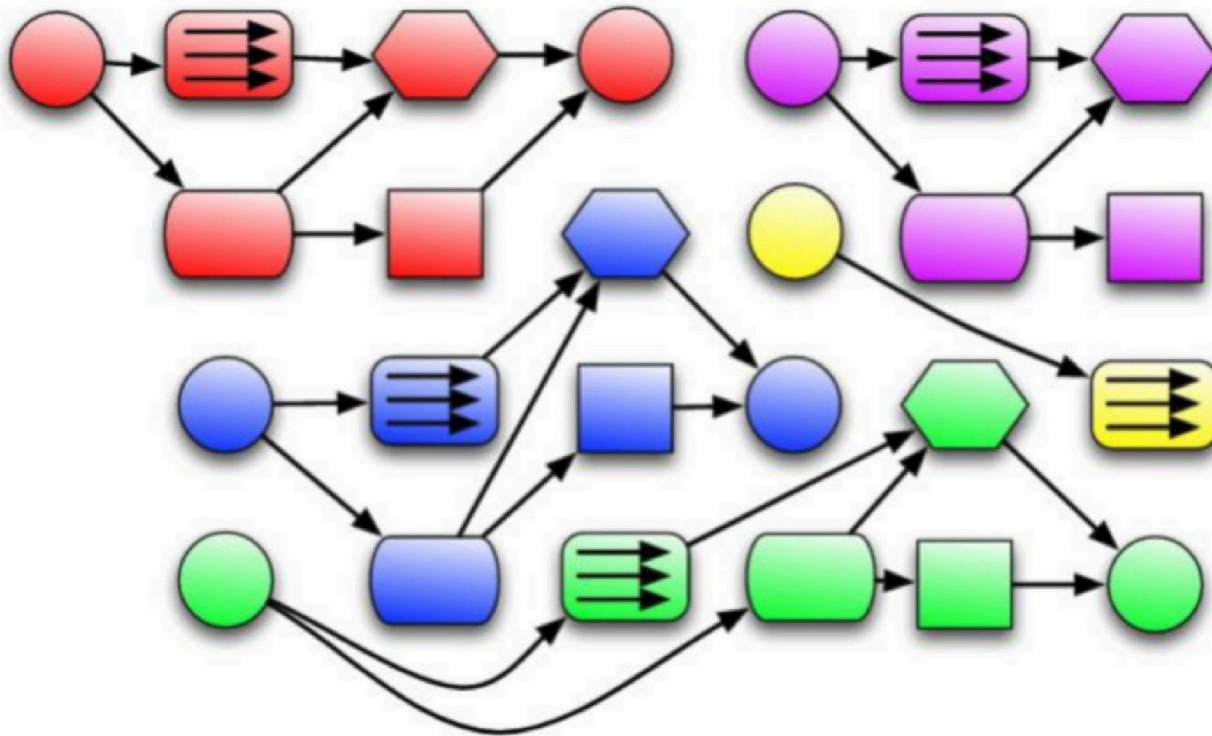
Figure 2: An example of multithreaded execution in AthenaMT. Four threads are shown, each corresponding to one row. Different events are shown with different colours, and different algorithms are shown with different shapes. The algorithms are executed as soon as their input data are available and a thread is free. (Image: ATLAS Collaboration/CERN)
